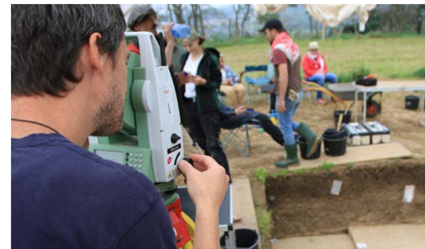
Step 1.2 (cf. Fig. 1): All marker positions are fixed by total station measurements.
