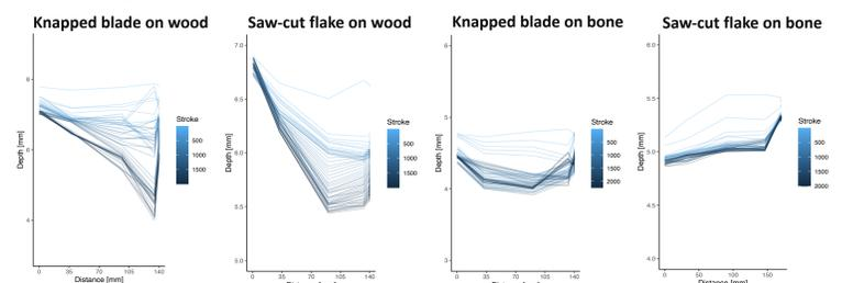
**Figure 2** Penetration depth of samples in their contact material throughout experimentation. Lines illustrate every 40<sup>th</sup> cutting stroke of the whole experiment—the darker the shade, the higher the stroke number.
