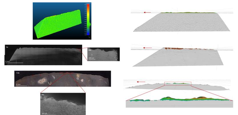
**Figure 1** Edge damage on sample FLT8-1 (top left) and contact areas calculated in the OFA software (top right). Polish and contact areas in OFA on sample FLT8-13 (middle) and FLT13-1 (bottom).
