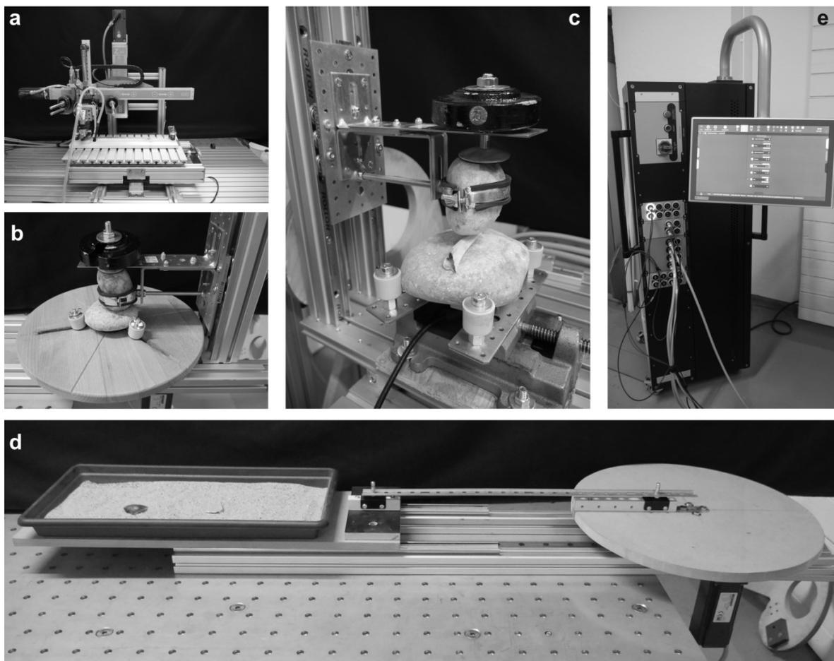
Fig.1: The SMARTTESTER® (inotec AP GmbH, Wettenberg, Germany) is a modular system that can perform several tasks in a repeatable way, including (a) cutting/scraping, (b) grinding, (c) pounding and (d) oscillation (back-and-forth). The controlling unit is shown in (e).
