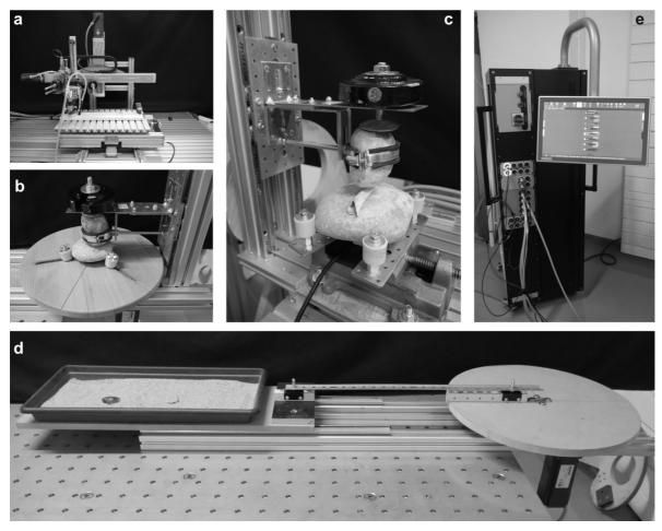
*Fig.1: The SMARTTESTER® (inotec AP GmbH, Wettenberg, Germany) is a modular system that can perform several tasks in a repeatable way, including (a) cutting/scraping, (b) grinding, (c) pounding and (d) oscillation (back-and-forth). The controlling unit is shown in (e).*
